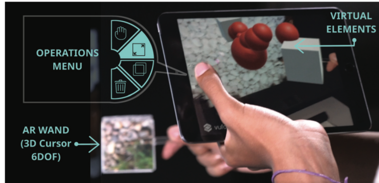
(b) Tangible wand to provide 6DoF in different modes based on selection in on-screen operations menu (Rodrigues et al. [2017]).
