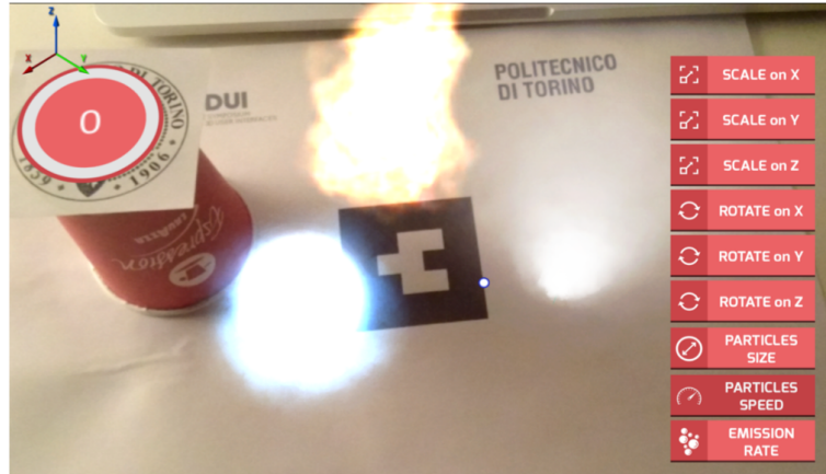
(a) Tangible rotary knob on the left to adjust one-dimensional parameter based on selection in on-screen menu on the right (Cannavò et al. [2017]).
