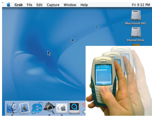
Figure 1. The sweep technique can be used to control a cursor on the large display like an optical mouse.
