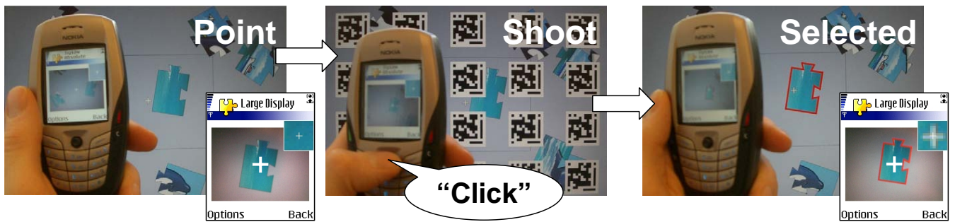
Figure 2. Point & shoot technique: (Left) The phone display is used to aim at a puzzle piece on a large display. (Middle) Pressing the joystick indicates selection and a visual code grid flashes on the large display to compute the target coordinates. (Right) The grid disappears and the targeted piece highlights to indicate successful selection.
