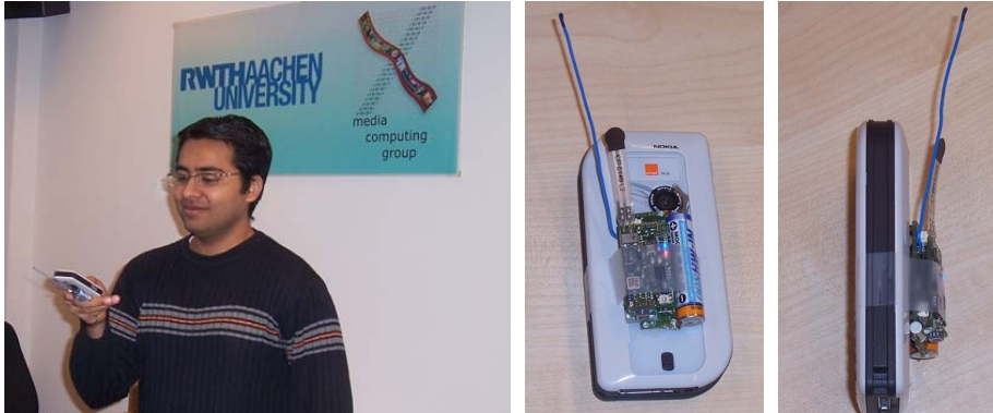
Fig. 1. (Left) A user testing a tilt scrolling interaction with the mobile phone as described in [8]. (Center & Right) back and side views of the mobile phone augmented with the Smart-Its particle board and sensor module. The module can be attached to the phone in whatever position the designer finds most appropriate.
