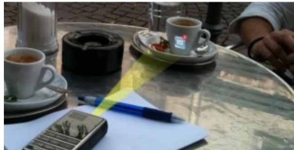
Figure 2.1: A pico projector used to project an interface onto an object, in this case onto a cup. Huber et al. [2012]
