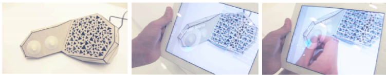
Figure 2.4: Left: A handicraft worked radio (TUI) / Middle: GUI is programmed with the help of tablet / Right: User manipulates the TUI and the changes are visible in the GUI. Heun et al. [2013]
