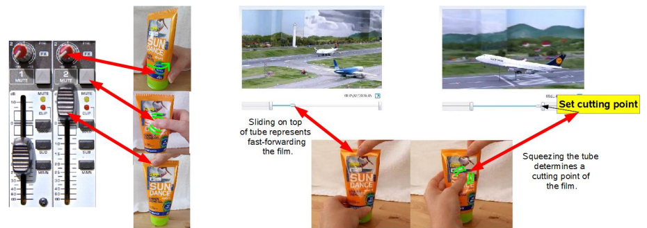
Figure 1.1: Left: Example of an everyday object that represents the affordances of physical controls. / Right: Example of how a tube could be used as controller to cut a film.
