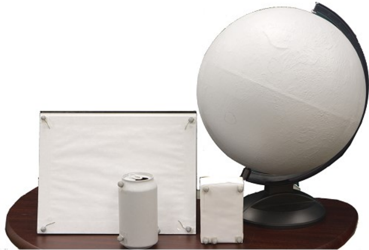
Figure 2.5: Physical models equipped with reflective markers of the Vicon motion capture system. Akaoka et al. [2010]
