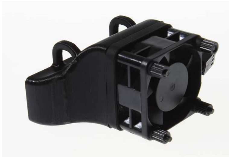
Figure 3.6: One of the four fans to cool down the surface.
