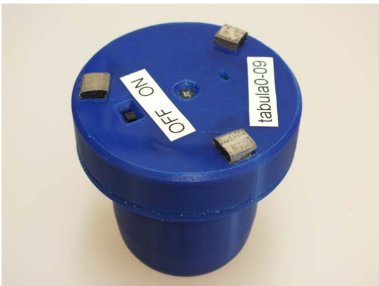
Figure B.5: Tangible from underneath, where the On/Off button and the soft pads (conductive EMS) are visible.
