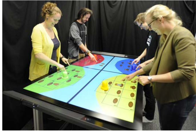
Figure 1.1: User standing at a tabletop playing a game in which tangibles are integrated into the interaction.
