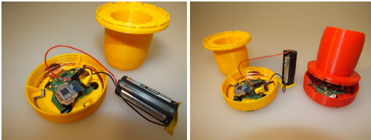
Figure 4.4: Left: Yellow tangible fully assembled. / Right: Yellow tangible ready to be fitted together with the upper part, Red tangible almost fitted together.
