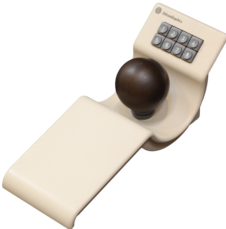
Figure 1.6: Example of a Spaceball input device manufactured by SiliconGraphics. The ball at the center of the input device can be pushed, pulled, and twisted to control up to six degrees of freedom, e.g., to move and scale 3D virtual objects. Like the isometric joystick, the Spaceball consists of strain gauges that capture the direction and the magnitude of the force applied to the ball. The keys (1–8) are used for accessing UI shortcuts. Image (slightly modified and resized) taken by Rama.
