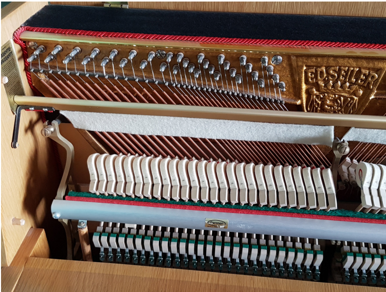
Figure 1.4: Close-up of the hammer mechanism found in pianos. When hitting a key, the hammer strikes a string such that a tone is generated. Depending on how strongly the player hits the key, the hammer will pluck the string differently: the more force is exerted on a key, the louder the tone will sound. In comparison to the harpsichord, the piano increases the player’s expressiveness since she can now also control the loudness of each tone. Image (slightly cropped and resized) taken by Sergej Medvedev.
