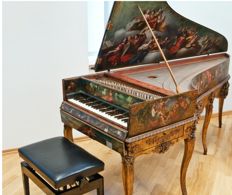
Figure 1.3: Setup of a harpsichord. The harpsichord consists of a keyboard that is connected to a set of strings on top of a resonating body. Hitting a key plucks a string such that a tone is generated and amplified via the resonating body. The force with which the player hits the key has no effect on the loudness of the generated tone. Image (slightly cropped and resized) taken by Sergej Medvedev.
