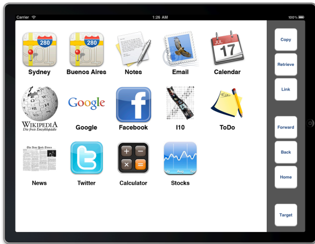
Figure 5. A screenshot of the iPad client's home screen. Operations are executed by tapping the appropriate buttons on the right. The button on the lower right is held to mark the client is the current target.
