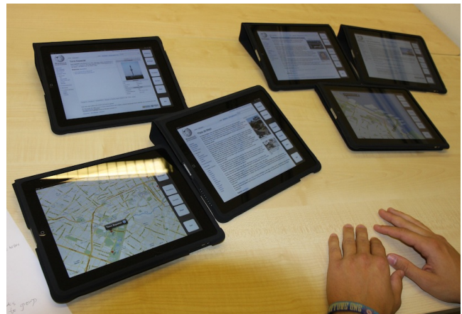
Figure 9. Arrangement of Tangible Windows for the planning task. Both groups of 3 Tangible Windows represent 2 sights, which are both shown in the opened Wikipedia articles. The markers on the map could be identified using the back and forward operation.
