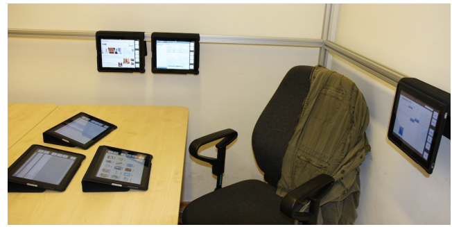
Figure 7. User setup of the workspace. The Tangible Windows on the desk show the Todo list, Mail, and the home screen; the Tangible Windows on the wall show News, Stocks, and the calendar.
