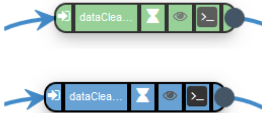
Figure 5.6: Nodes from the high-fidelity prototype that are in a state of execution. The code of the green node is executing. The blue node waits for inputs from other nodes.
