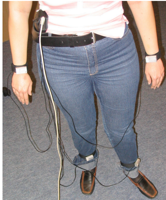
Figure 2.2: RST's acceleration sensors attached to a person. The actual attachment is achieved using velcro fasteners, the USB hub is worn mounted on the person's belt.
