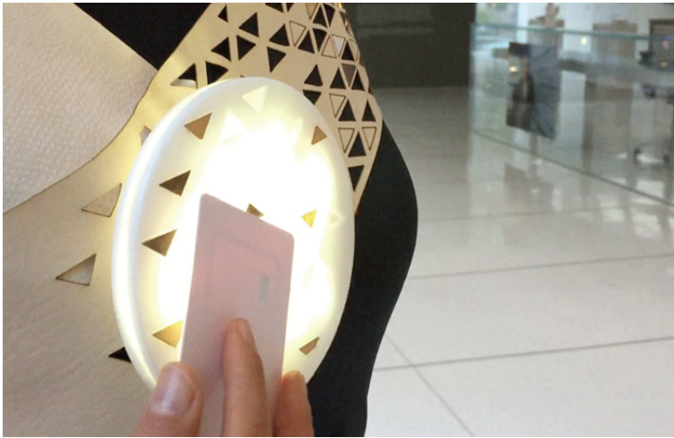
Figure 2.3: Picture of the wearable Motif artifact, when in contact with a RFID chip. By Druga et al. [2017].
