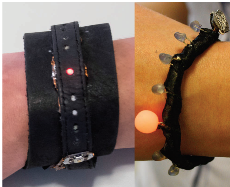
Figure 2.4: Picture of the WaterJewel Bracelet prototypes for male (left) and female (right) users. By Fortmann et al. [2014].
