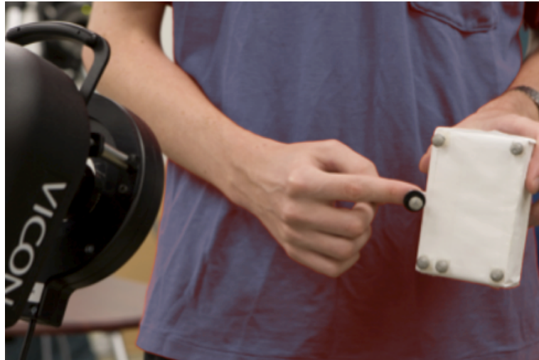
Figure 2.4: A physical prototype made out of Styrofoam with retroreflective markers is used with the DisplayObjects toolkit. The markers are attached to enable a Vicon system to capture its location, orientation and deformation. A 3D model of the prototype is used to project an interface onto the object's surface. Another marker on the user's finger is used to interact with the interface.
