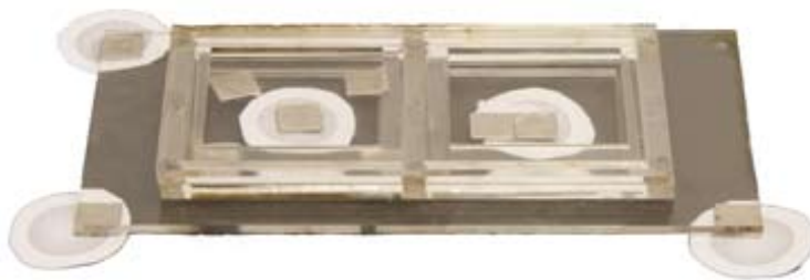
Figure 3.2: Photo of a radio-button Madget with two buttons. To be able to elevate the button plates there are magnets attached to them. The markers on the plates allow to check if the actuation succeeded.
