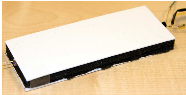
Figure 2. The smaller hardware prototype to measure horizontal bending. The dimensions are about 13 cm x 5 cm.
