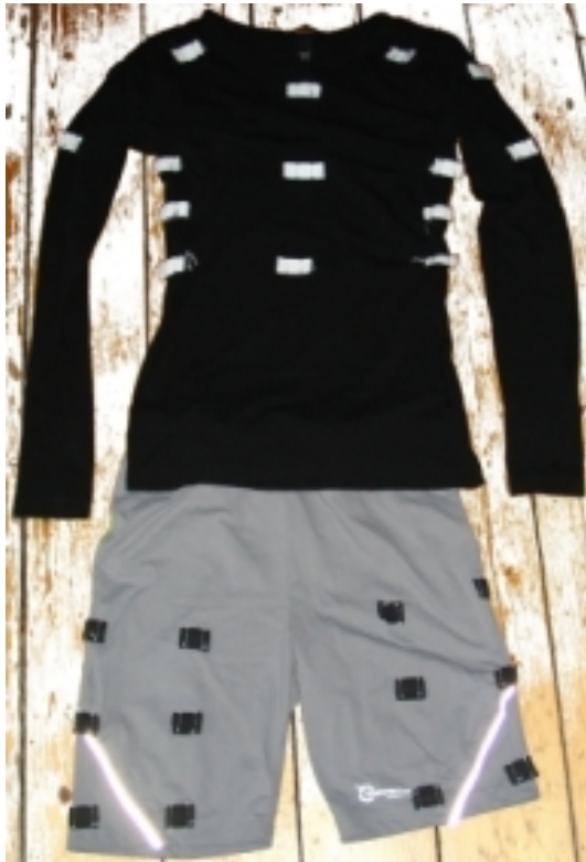
Figure 4.10: Tight-fitting shirt and short with loops to add the vibration motors
