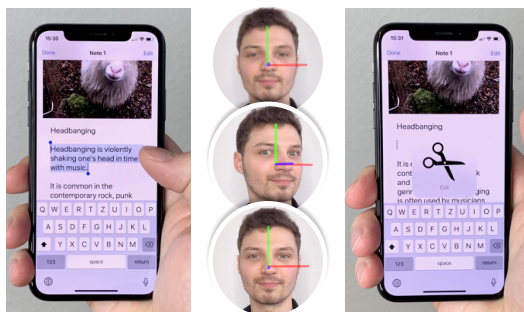
Figure 9: In this example, the user selected a part of the text that he wants to cut. After selecting the text with his finger (left) he performs a Handbang gesture to the left (middle) to cut the text (right).
