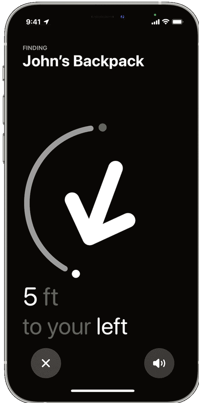
Figure 1.2: Precision finding of an AirTag shows the direction as well as the distance precisely and adds vibrations the closer the user gets to the AirTag 11 .
