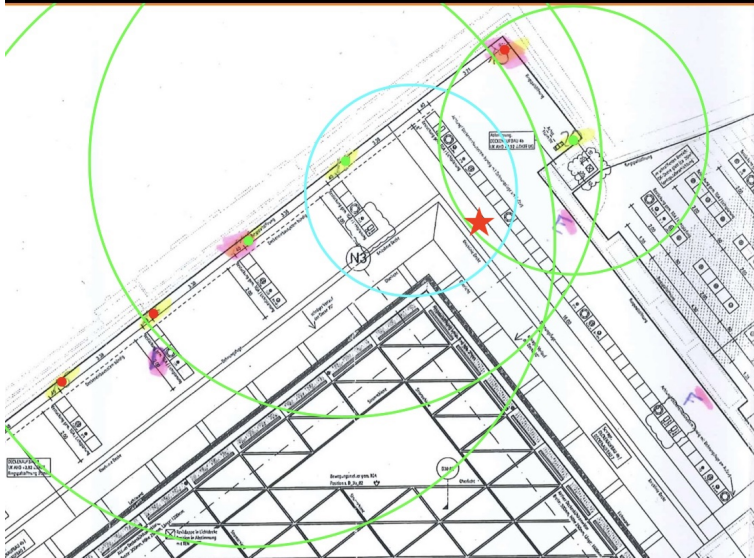
Figure 5.1: Average positioning in a corner of the triangle that is the Centre Charlemagne museum. The code automatically detected a non-linear alignment of the received beacons and decided to fallback to averaging. The red star shows the actual position the screenshot was taken at.
