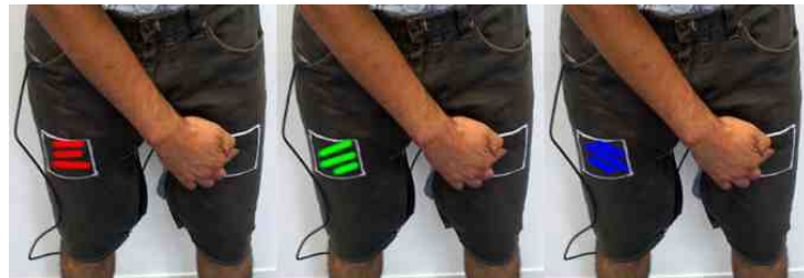
Figure 8.2: Variance in the orientation of gestures articulated on thigh. Left image shows articulations parallel to the sensor's horizontal borders, and remaining two images depict varying degree with respect to them.
