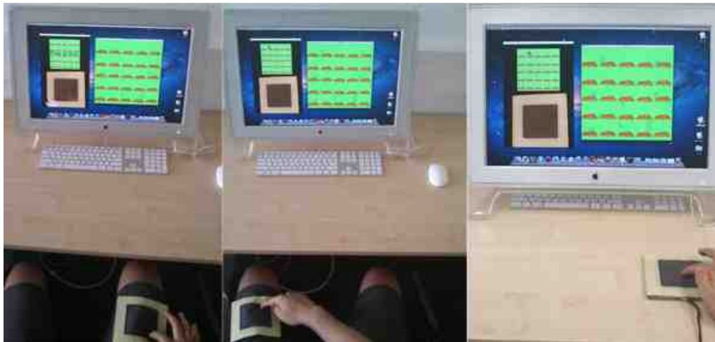
Figure 6.4: Setup for target acquisition study. Left and middle images depict prototype attached to thigh and the right one when it is placed on the desk.
