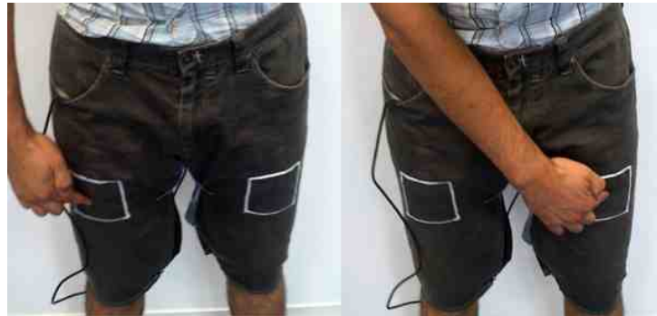
Figure 5.5: GestiPants worn. The two images illustrate that articulation with the same hand on both sensors is possible.
