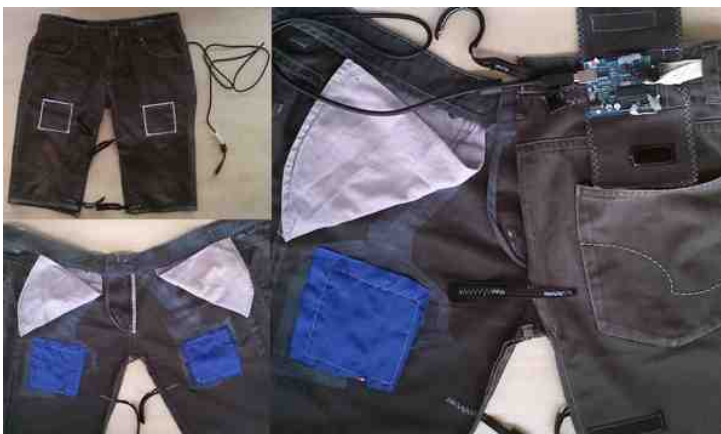
Figure 5.4: GestiPants - pair of jeans with a sensor embedded in each leg. Left images show the two sensors and right one - the microcontroller placement and insulation.
