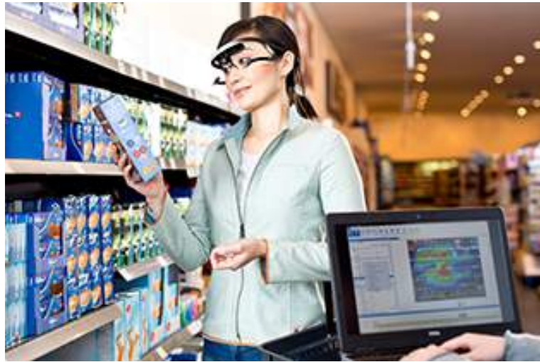
Figure 3.5: This picture shows an application example for a mobile head mounted eye tracker. This device records the eyes with two cameras placed directly in front of them and computes the gaze direction based on the location of the pupil. [ https://www.ergoneers.com/en/newsroom/applications/ (27.07.2018)]
