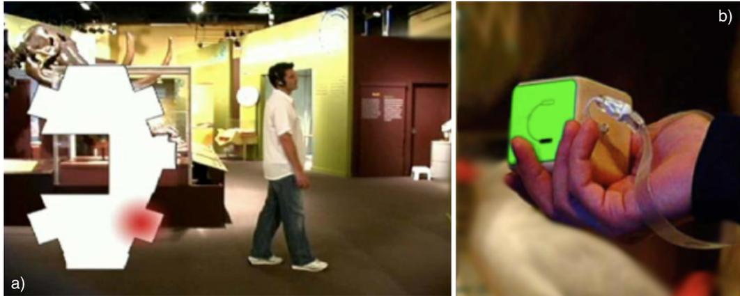
**Figure 2.1:** a) A visitor walking through an exhibit room. On the left hand one can see a room map, the red gradient depicting the volume of an ambient sound, heard when being on the map position. b) The tangible user interface. (both figures taken from Wakkary and Hatala [2007])
