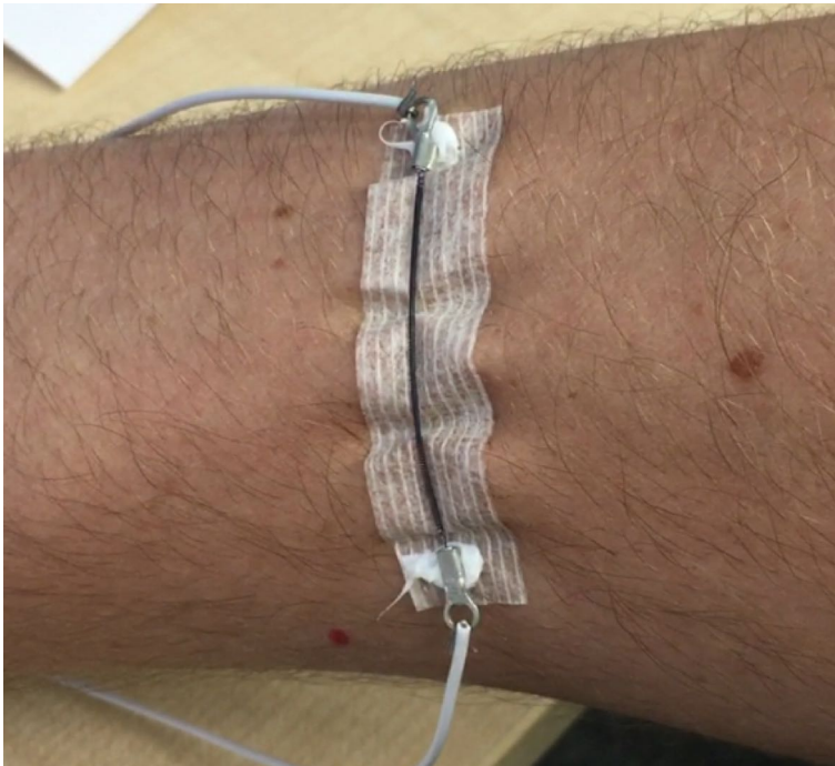
Figure 3.2: A pilot haptic prototype based on a single BMX in the contraction phase.
