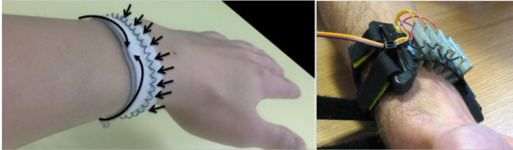
Figure 2.2: Haptic devices based on SM actuators. From left to the right: Gupta et al. [2017] , squeezing, SMA; Knoop and Rossiter [2015] , stretching, SMA.
