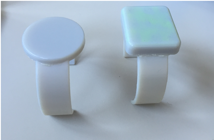
Figure 3.1: 3D printed prototypes used for the test. The dimensions match the commercially available smartwatches.
