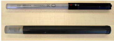
Figure 4. Buchla Lightning II digital batons. The baton on the top is the original baton, made from aluminum and fiberglass. The baton on the bottom is our repackaged version of the baton made from plastic and resin for better durability.
