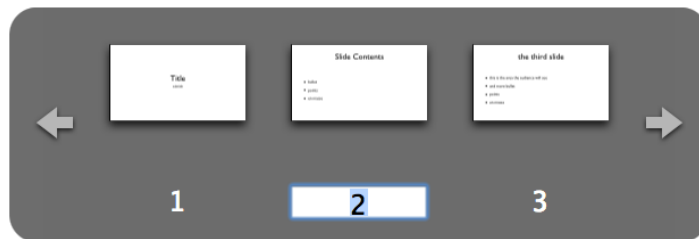
Figure 2.3: Apple Keynote's slide switcher: the presenter can select a slide in private with the arrow buttons or by typing the slide number. She confirms the selection by pressing ENTER.
