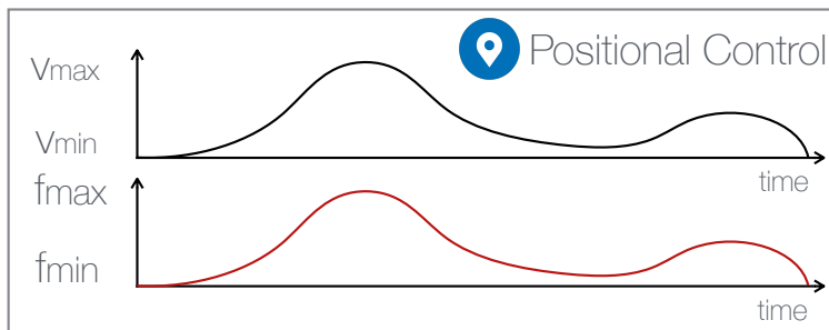
Figure 4.1: Positional Control: value and force correspond to each other [IOSTE, 2016].
