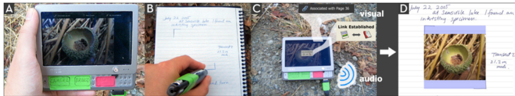
Figure 2.9: ButterflyNet: augment the notebook by associating the picture to specific position on the paper.
