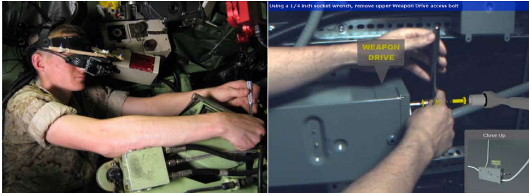
Figure 2.2: (Left) A mechanic wearing a tracked HMD performs a maintenance task. (Right) AR condition in the experiment shows localized labels and 3D models as instruction.
