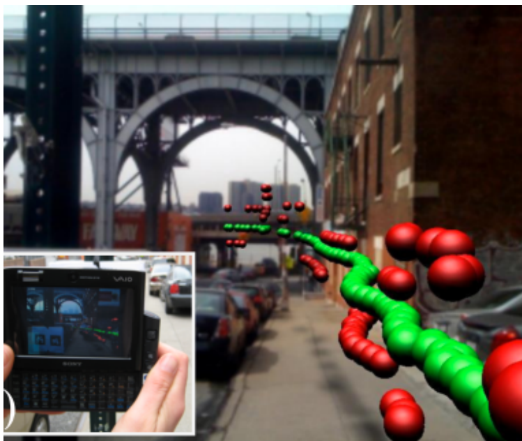
Figure 2.8: SiteLens: visualize geocoded carbon monoxide data in AR scene for urban designer.
