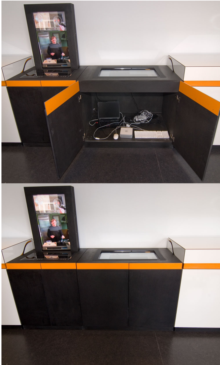
Figure 7.6: On the left side: The open kitchen element reveals the hardware. On the right side: Closing the kitchen element hides all internal hardware.
