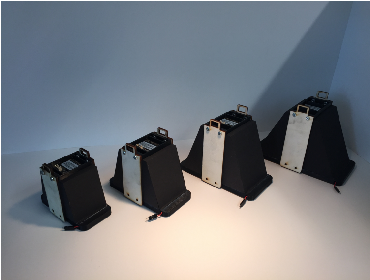
Figure 3.13: Picture of the assembled final prototypes. The cable that comes out of the lower part of each prototype is connected to the LEDs and can be plugged to a power supply. From left to right: Prototype A , Prototype B , Prototype C , Prototype D .
