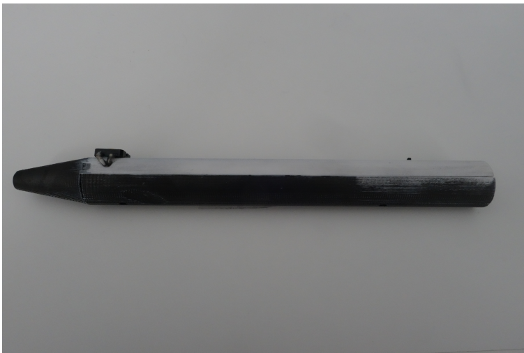
Figure 3.4: The 3D-printed hull of the Pengible. The black parts are coated with a thin layer of graphite.
