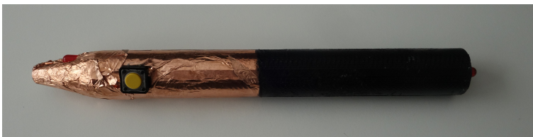
Figure 4.1: The Pengible version used in this study, equipped with two LEDs, two vibration motors and one button. (For the study the red LEDs were exchanged with multi-colour LEDs). A dent on the back lets the Pengible rest more comfortably in the hand while holding.
