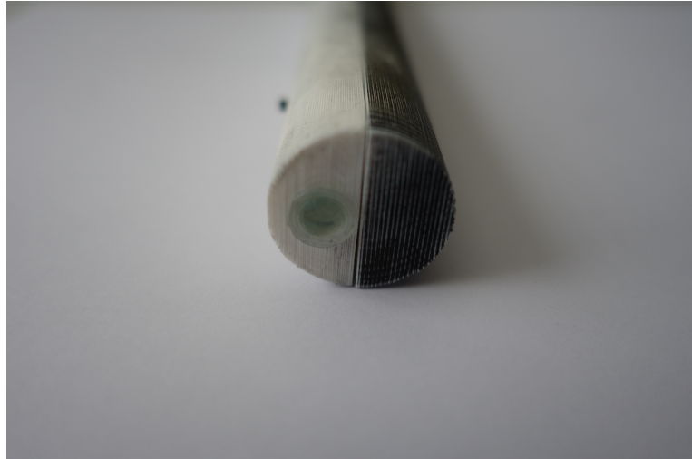
Figure 4.8: Diffuser for the back LED made from translucent material
