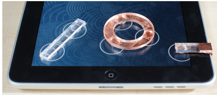
Figure 2.3: PUC widgets on an iPad: a transparent Bridge PUC (left) and a Ring PUC (center). The clip to permanently ground a touch point and override the iPad’s adaptive filter can be seen on the right. [Voelker et al., 2013]
