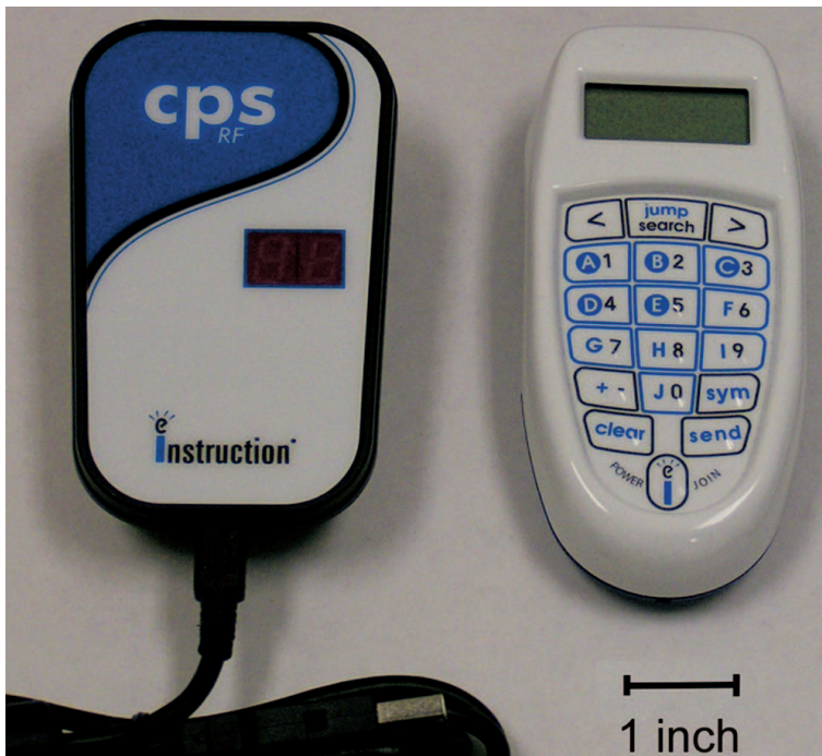
Figure 2.1: Classroom Performance Keypad (right), with which students can answer questions or polls and Clicker Receiver (left) which can wirelessly collect data from all keypads [Barber and Njus, 2007].
