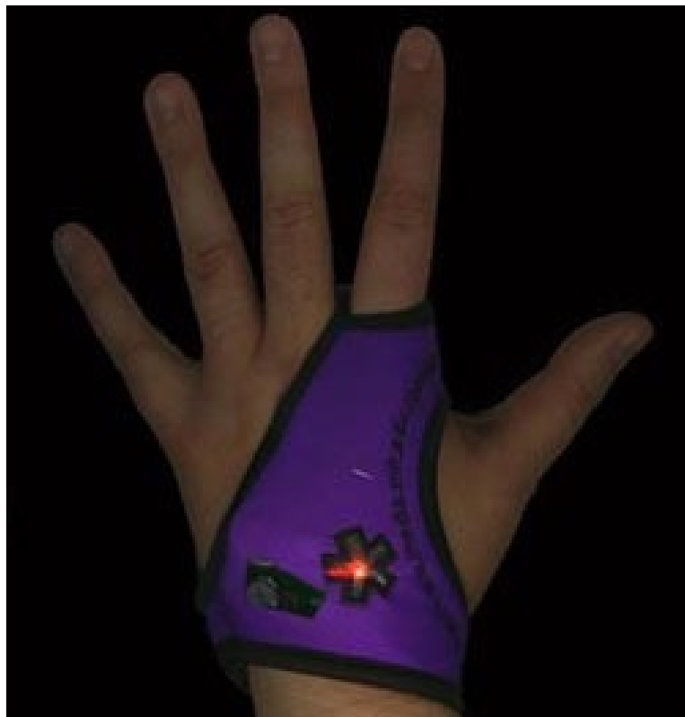
Figure 2.3: The glove of the Galvoactivator [Picard and Scheirer, 2001].
