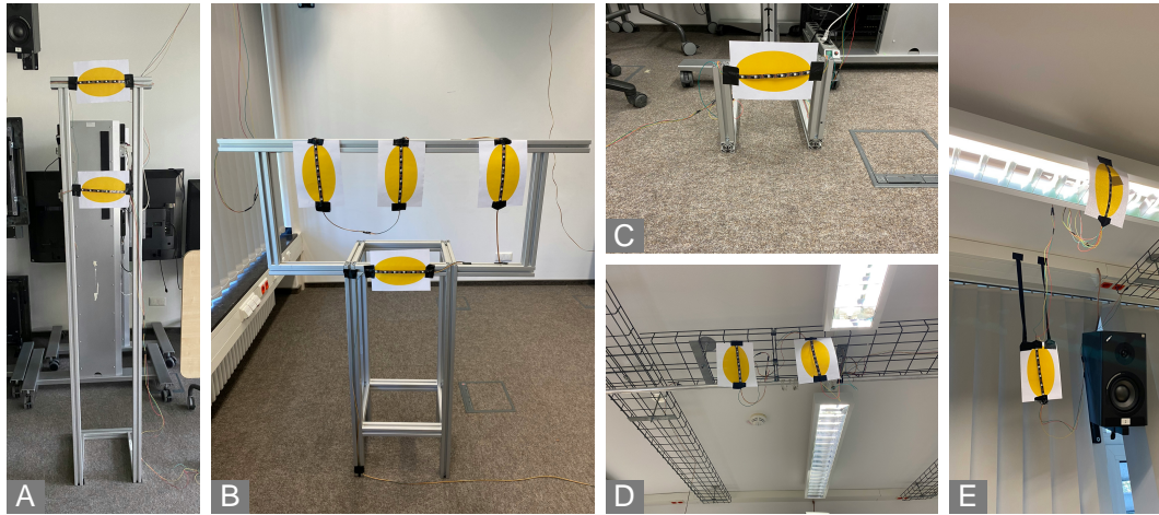
Figure 3.10: Aluminum extrusion constructions were used to distribute targets across the room. Other targets were taped to the ceiling. Construction A represents a floor lamp with two light bulbs, B represents a lamp with three bulbs above a table that has a controllable device placed on top. Construction C represents an LED strip near the ground, D a ceiling lamp with two light bulbs, and E represent blinds in the back with a ceiling light in front.
