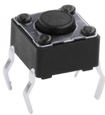
DTS61K button that is used in all button-based controllers.
