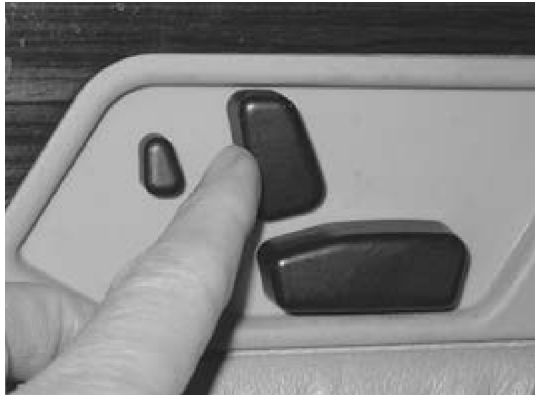
Figure 2.7: Seat adjustment in a Mercedes-Benz. The control resembles the device it controls, making the interaction with it intuitive. Image taken from Norman [2013].
