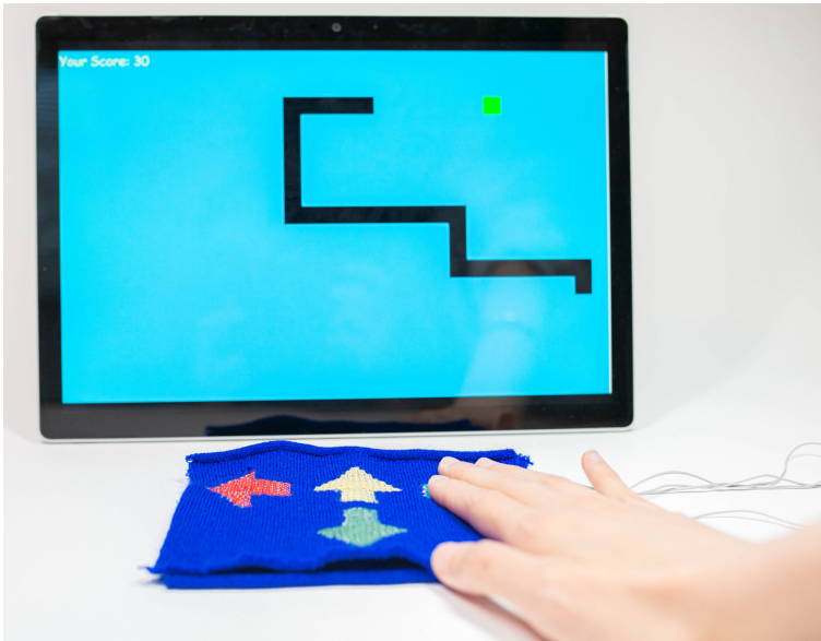
Figure 2.3: A knitted controller created with the techniques proposed by Luo et al. [2021] that is used to play snake on a connected computer.
