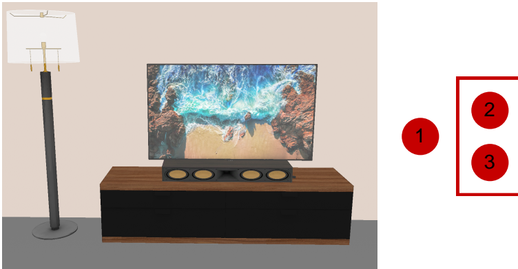
Figure 3.3: Example mapping of the Cluster Map showing how a floor lamp (button 1), TV (button 2), and speaker (button 3) are mapped to the controller.
