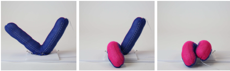
Figure 2.4: Textile V-shape with integrated tendons as proposed by Albaugh et al. [2019]. Both legs of the V can be moved independently by pulling at the attached strings.
