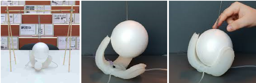
Figure 2.1: Two movements of the helpless soft robot, gripping and reaching. Human collaboration is needed.
