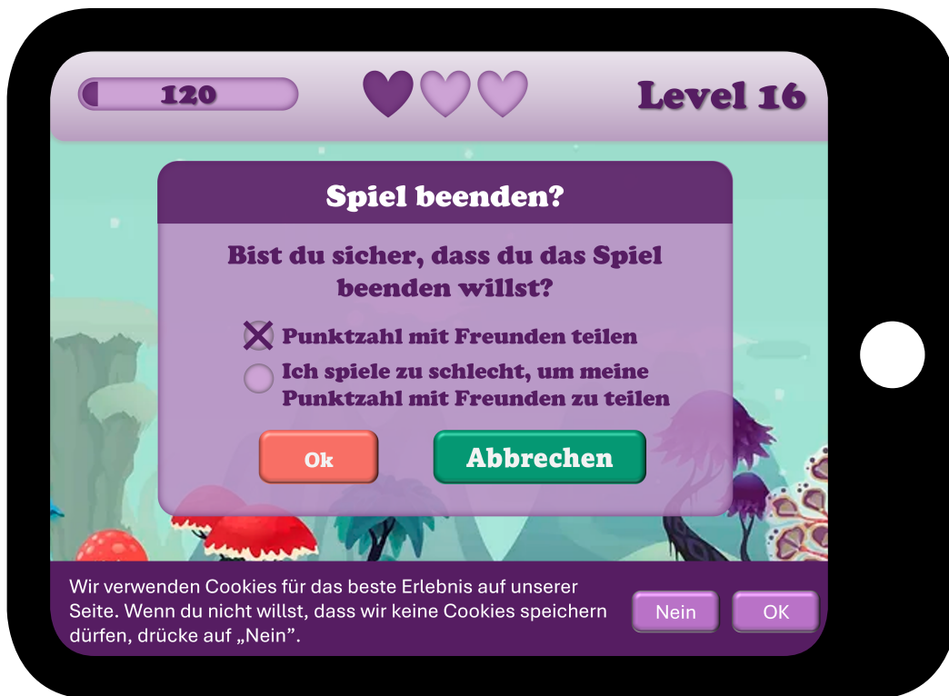
Figure 3.3: The design for the recognition task in Part 3 contains four dark patterns: 1) Toying with Emotions: the user is asked if they are sure they want to leave the app, with one ‘Ok’ button in red (left) and one ‘Cancel’ button in green (right). 2) Preselection: the checkbox for sharing the score with friends is preselected. 3) Confirmshaming: the formulation for the option to reject sharing the score is uninviting to select. 4) Trick Question: the cookie banner at the bottom of the screen uses double negations.
