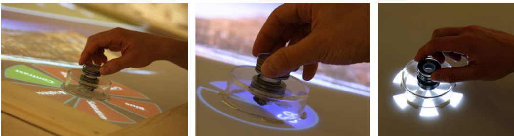
Figure 2.4: Acrylic rotary SLAP widget (by Weiss et al. [2009]) on an acrylic surface.
