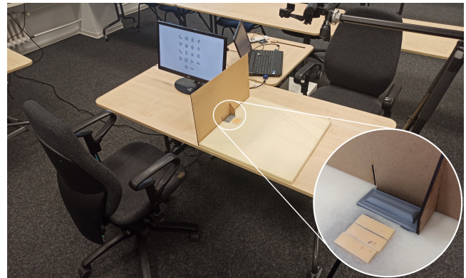
Figure 3: The setup from our user study: A monitor was placed in front of the participant to show digital versions of the tested shapes. Behind a sight protection, Velcro was placed on the padding foam to fix the icon's location during the task. The button was used for time measurements and the participant's hand was video recorded during the trials.
