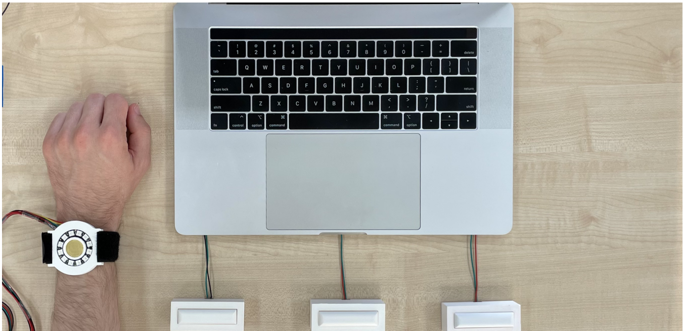
Figure 1: Our wrist-worn prototype supplied presenters with additional visual, haptic, or auditory cues during online presentations to raise awareness of incoming notifications from the audience without disturbing the presenter's flow. Our study participants had to recognize three different types of Zoom notifications and press a corresponding button while giving a presentation.
