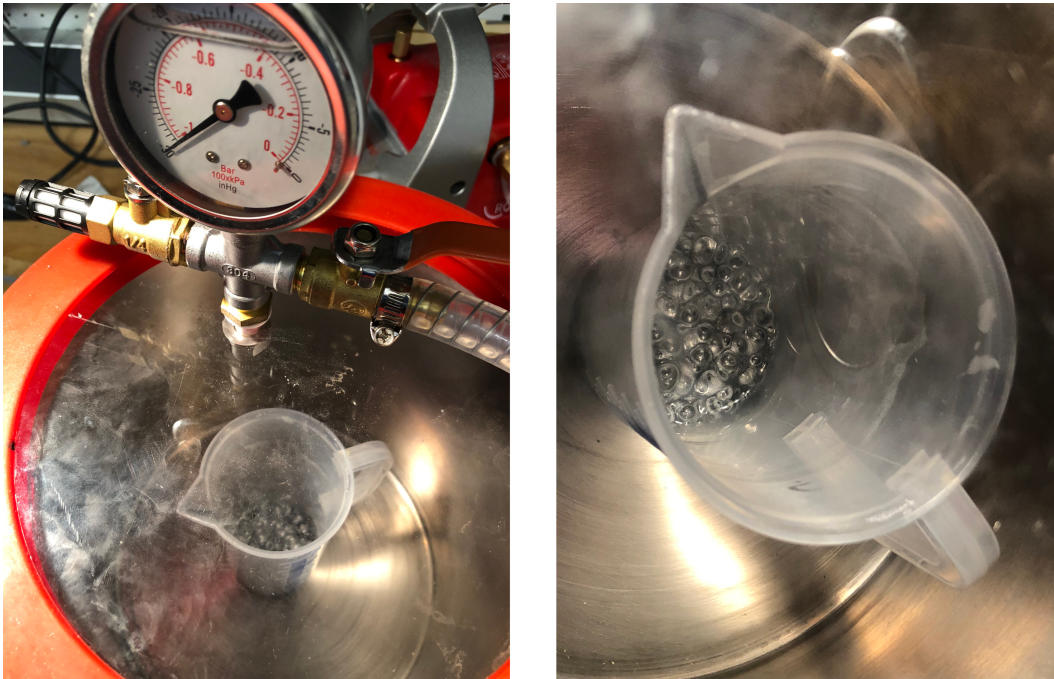
Figure 3.9: To degas the mixed silicone, it was vacuumed with -1 Bar ( left ) until it boiled ( right ) and left for one minute until almost no more bubbles popped on the surface.
