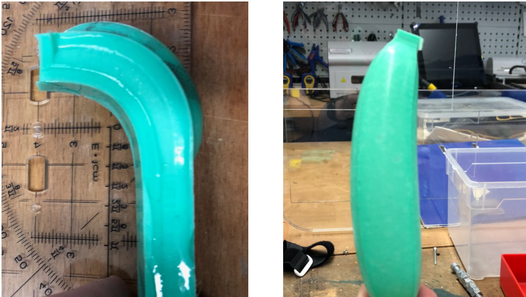
Figure 3.2: Soft robots created with the SoRoCAD approach have faced issues. Actuators could perform a bend but showed a bulge at the outer side ( left ). At the same time, the trials of creating an elongation movement ended in banana-shaped balloons ( right ).
