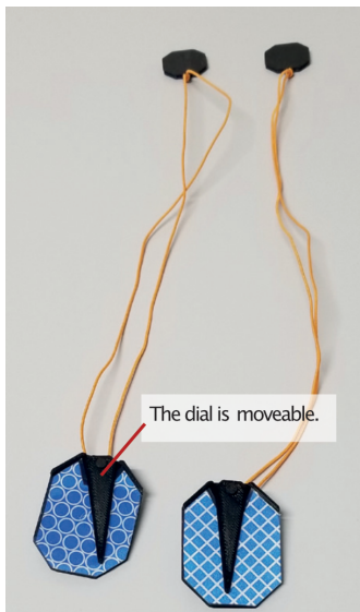
Figure 2.4: Picture by Jarusriboonchai et al. [2020] showing the multi-wear pins that can be used to communicate the wearer’s own emotional state to the partner’s pin through rotation of a dial
