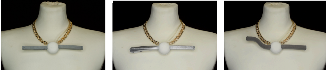
Figure 4.3: The necklace shown to the participants consists of a golden chain that holds a pendant. Two soft robots fit into the sides of the 3D-printed pendant ( left ). The left soft robot could change its shape by being actuated with compressed air. By changing the soft robots and their covers, diverse shape changes can be realized ( center & right )
