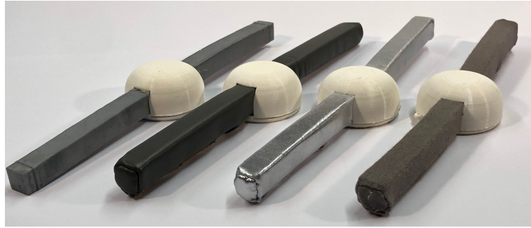
Figure 4.1: The surface material of the soft robots used in the necklace was either silicone , leather , metal , or fabric (from left to right). Each participant in the user study was assigned one of the four materials.
