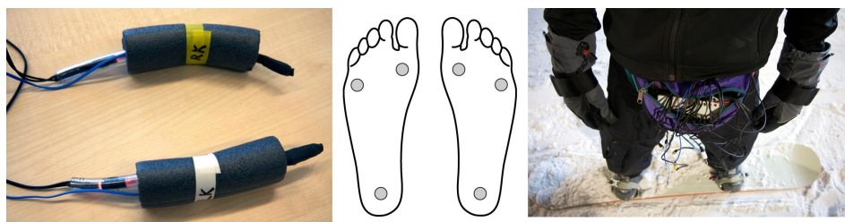
Figure 4.10: Left: Optical bend sensors are robust and exhibit a linear response to flexion. The layer of foam shielded and fixated these sensors at the back of knees. Middle: Three force sensors captured the weight distribution. Right: The participants wore the SensAct box in a pouch.
