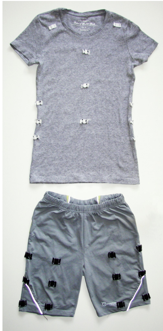
Figure 6.4: The first design of the tactile suit. Vibration motors were placed inside small pouches that were sewn on the fabric.
