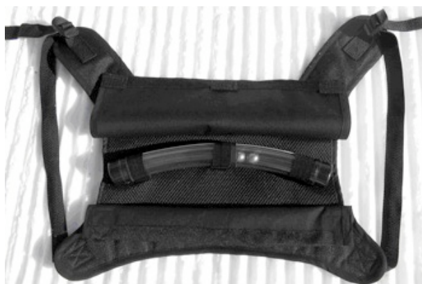
Figure 1.2: The Ski Coach [Braisby, 2005]. The clink of balls signals that the posture of the shoulders is correct (courtesy of Chris Braisby).
