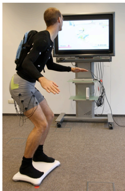
Figure 6.8: The cognitive and physical workload condition of the experiment required the participants to respond to tactile motion instructions on the Wii balance board. The actuator boxes were placed inside a backpack.
