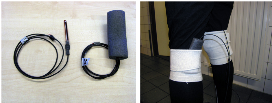
Figure 4.5: Elastic supports fixated bend sensors at the back of the knees to measure the amount of knee flexion during the ride.
