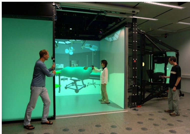
Figure 3.12: Photograph of the CAVE at the RWTH Aachen, which can be used to simulate virtual environments
