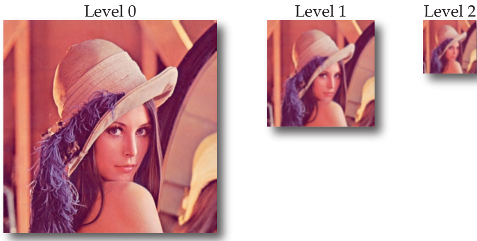
Figure 2.5: Different resolutions of an image pyramid, which is used to speed up the matching algorithm
