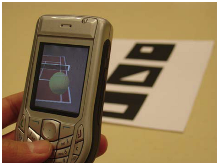
Figure 3.1: Scene from the AR Tennis project where a marker is used to determine the position of the mobile phone, from Henrysson et al. [2006]
