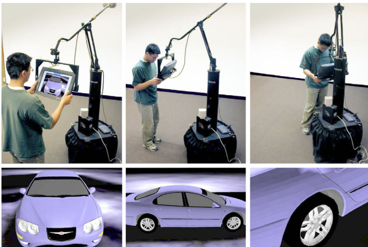
Figure 3.7: With the Boom Chameleon the user can navigate around the 3D model and place comments, from Tsang et al. [2002]
