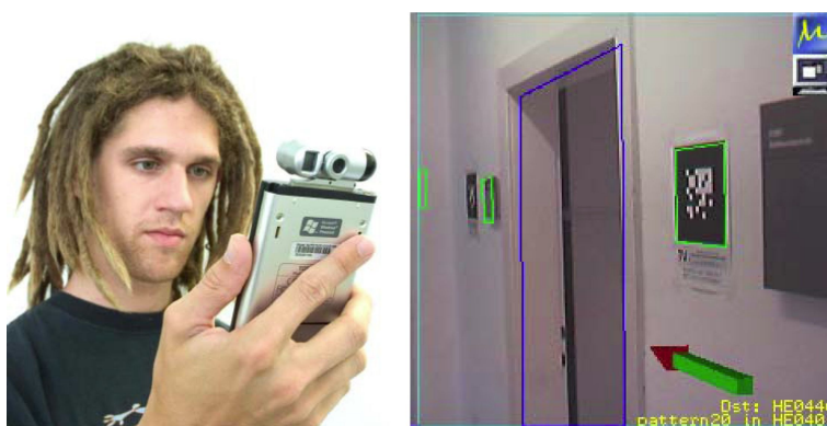
Figure 3.2: Screenshot of the guidance system by Schmalstieg and Wagner [2005] which uses fiducial markers
