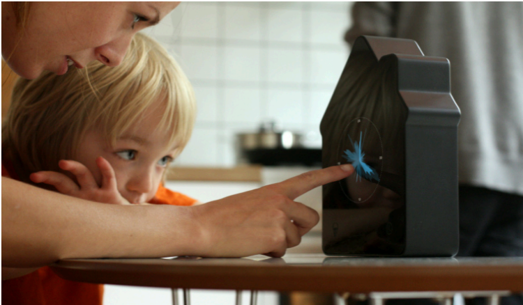
Figure 2.5: The EAC uses the clock as a metaphor to visualize historic and current data of energy consumption information in a visually pleasing object
