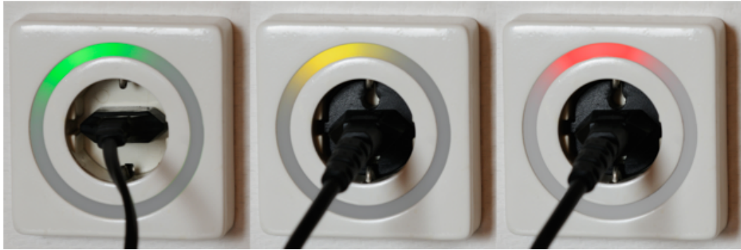
Figure 2.4: PowerSocket increases the awareness about energy consumption through a rotation animation that changes colors
