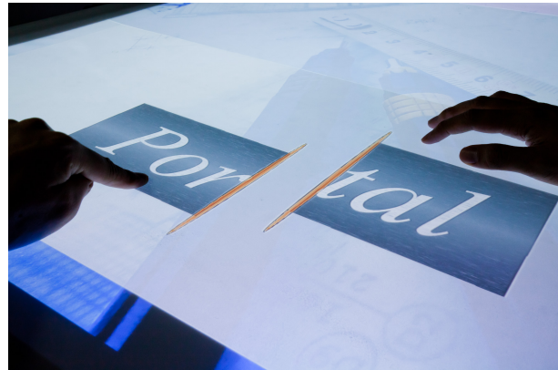
Figure 1: Dynamic Portals is a light-weight technique to exchange digital documents on interactive surfaces.
