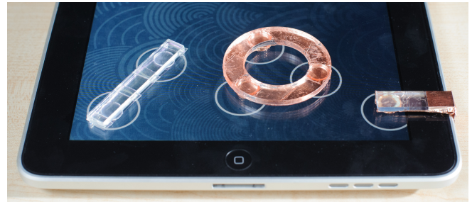
Figure 1. PUC widgets on an iPad: a transparent Bridge PUC (left) and a Ring PUC (center). The clip to permanently ground a touch point and override the iPad's adaptive filter can be seen on the right.
