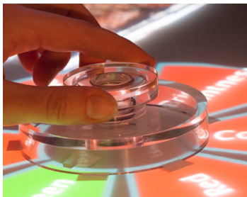
Figure 4: The SLAP knob [12] is a rotary button that can be pushed to confirm input.
