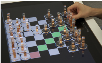
Figure 5: 1-Touch example: By touching a chess piece, the user is shown where he can move the playing piece (green squares) and where the piece can be hit by his opponent (red squares).
