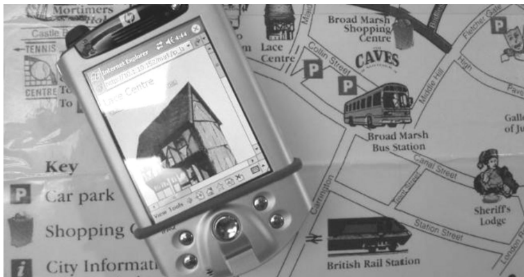
Figure 2.11: An old handheld device used as magic lens over a physical map. The device screen shows details of the attraction when being moved close to its location on the map. [Reilly et al., 2005]
