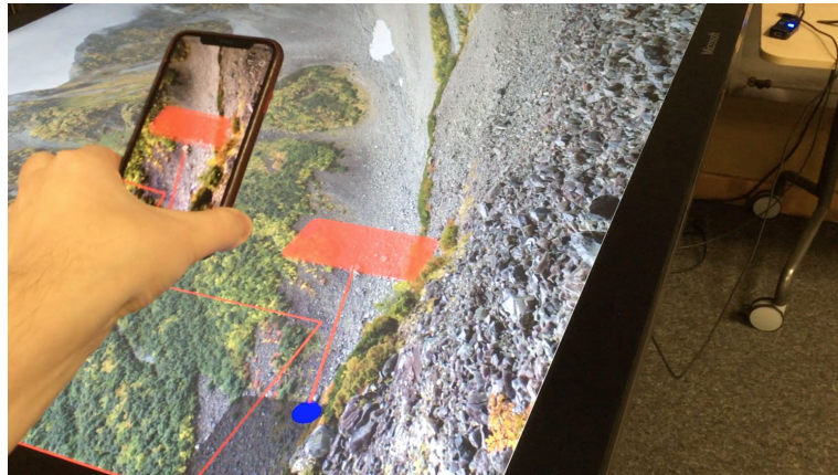
Figure 3.6: Raycast of the device’s viewfinder onto the tabletop surface: The device representation can be seen at the bottom, with a blue circle at the camera position. A red line indicates the raycast from the camera to the tabletop surface, where a red rectangle highlights the part of the content that is currently in the focus of the device. When looking at the device screen, this can be verified by checking that the red rectangle indeed is in its centre. (The red outline indicates which marker is currently tracked by the device.)
