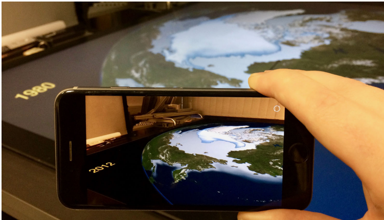
Figure 4.3: The iOS app uses parts of the 1980s picture as marker for ARKit’s image recognition and then calculates the correct size and position for the overlaying image from 2012.
