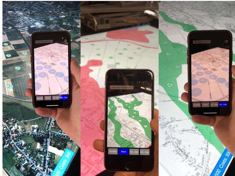
Figure 4.6: Users can explore multiple data layers to decide on windmill positioning by combining the tabletop layer (in the background) with different layers on their devices.
