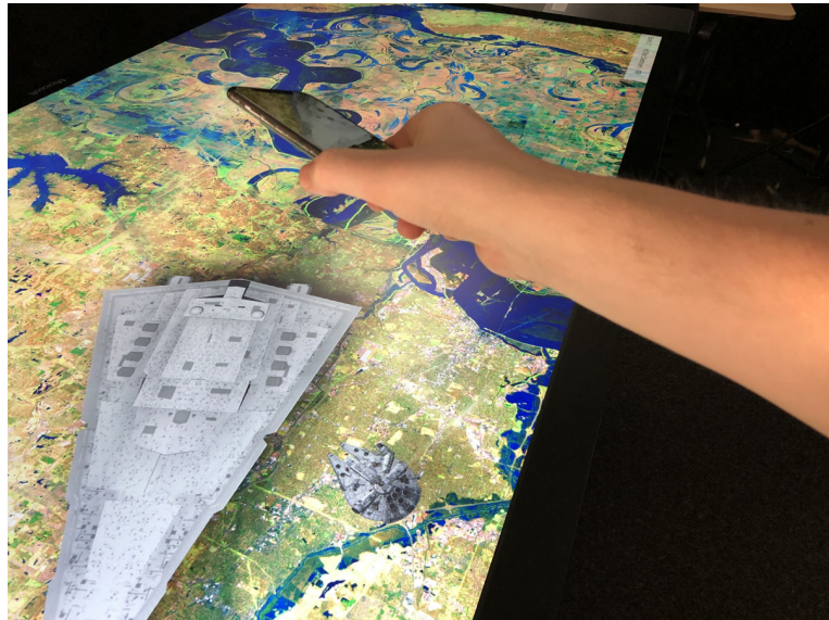
Figure 4.5: We implemented a direct mapping between the device and the virtual spaceship (the smaller one on the right). When moving, tilting or rotating the device, the virtual object behaves accordingly and with delay.
