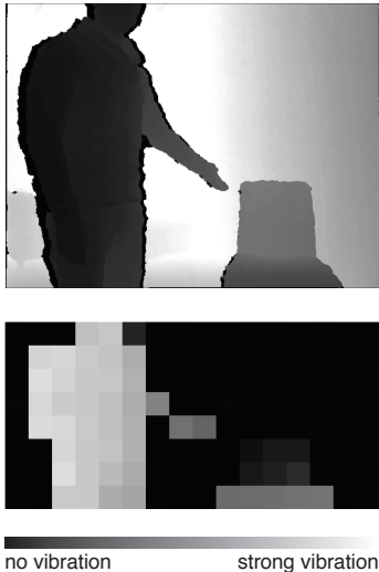
Figure 2: The depth image (top) is mapped to vibration levels (bottom). Closer objects produce stronger vibration. In this scenario, the gradient of vibration represents the tilted body of the person in front of the camera.
