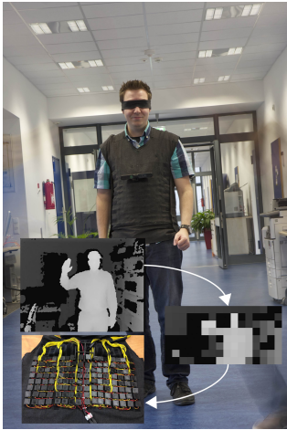
Figure 1: Depth information from an object is displayed as a vibrotactile image on the abdomen.
