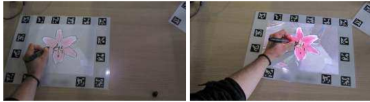
Figure 2.7: Drawing over a projection of a 3D model in Pa-pARt. (Image taken from Laviolle and Hachet [2012])
