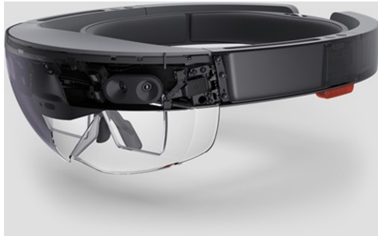
Figure 2.9: The Microsoft HoloLens is a head mounted AR device. (Image taken from Microsoft)
