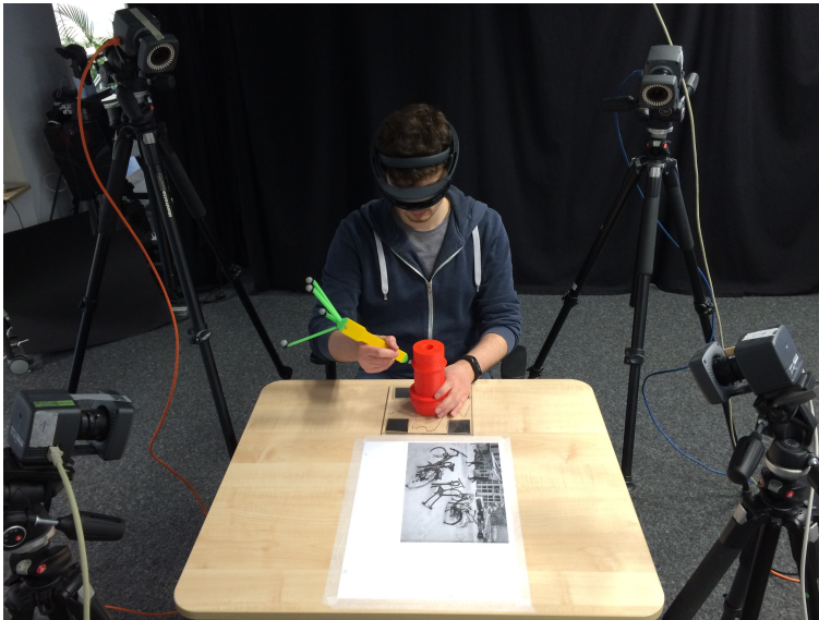
Figure 5.1: The table used in the user study surrounded by Vicon cameras. The visual marker and mounting on the table can be seen.
