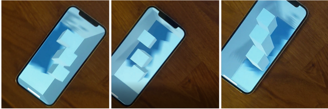
Figure 3.3: A depth illusion effect created by rendering the virtual scene from the perspective of the user.
