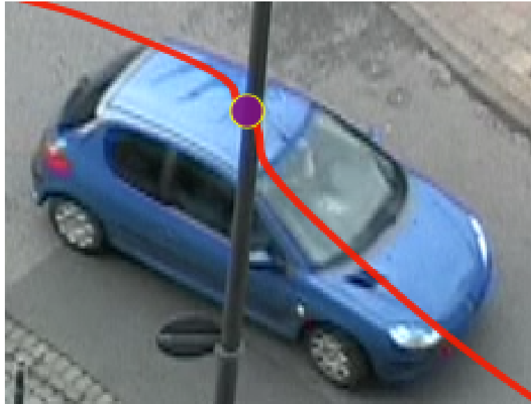
Figure 5.2: Resolving occlusion in DRAGON: When clicking on the streetlight a trajectory fitting the car is computed. This helps to resolve occlusions, when a motion vector of the car ends on the street light.
