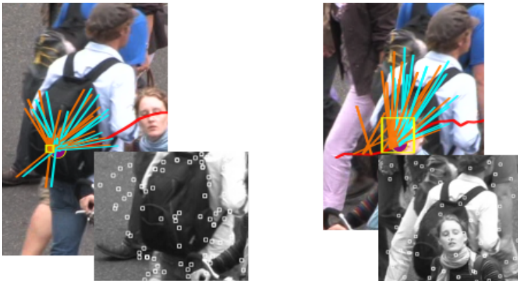
Figure 6.18: Backpack — Occlusion Handling: Two detail views from the backpack scene, the features used for tracking and the cutout used for detecting possible object features
