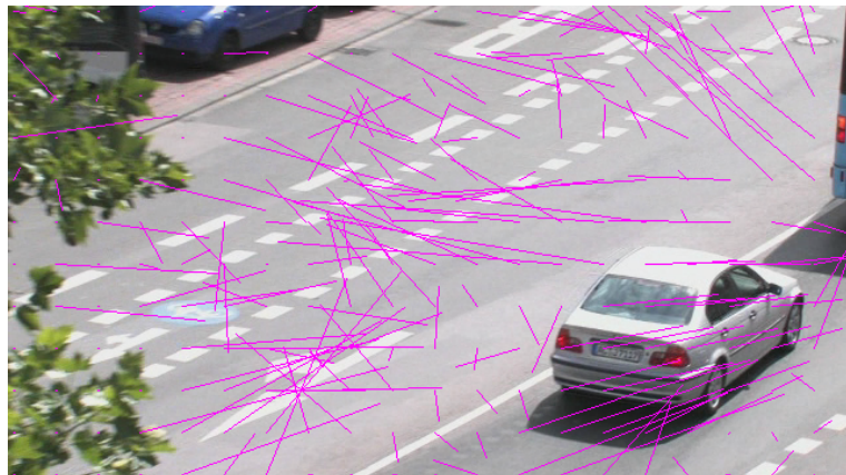
Figure 4.6: Unsuitable MPEG motion vectors: Motion vectors not fitting the camera motion. Extracted from MPEG4 encoded video
