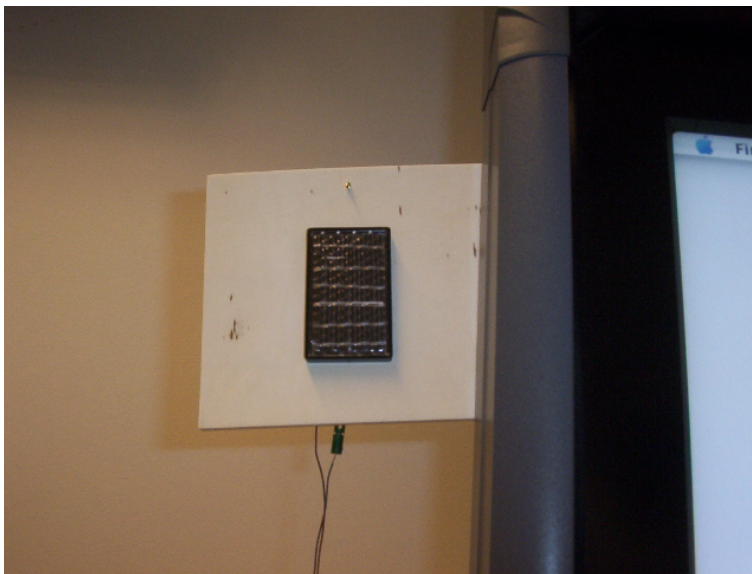
Figure 6.1: Solar cell attached to the upper-left corner of a plasma display.
