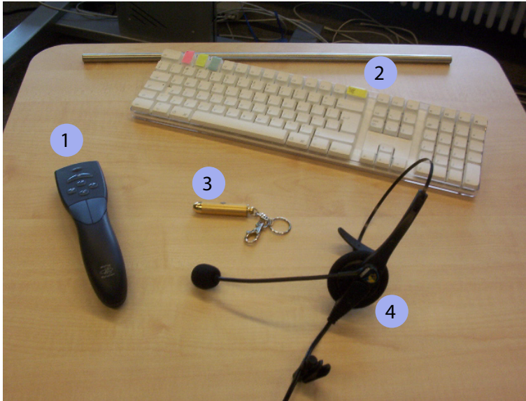
Figure 4.3: Input devices that we used: 1) gyro mouse, 2) wireless keyboard, 3) laser pointer, and 4) head-mounted microphone.
