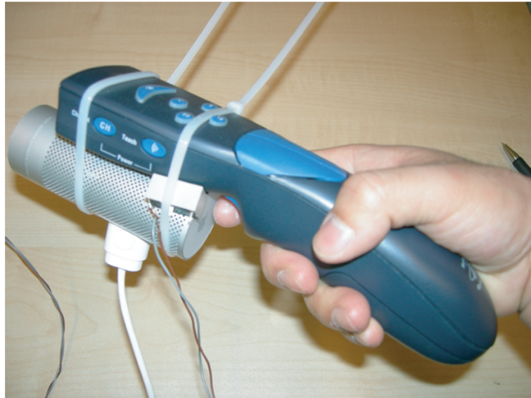
Figure 8.2: Focus device prototype with a coil driven switch.
