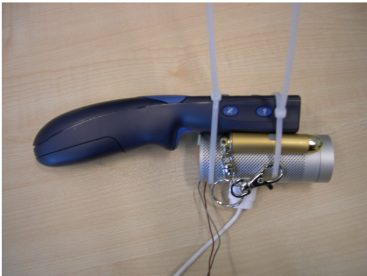
Figure 8.1: Focus device prototype consists of a gyro mouse, a webcam, a laser pointer and a magneto mechanical switch.
