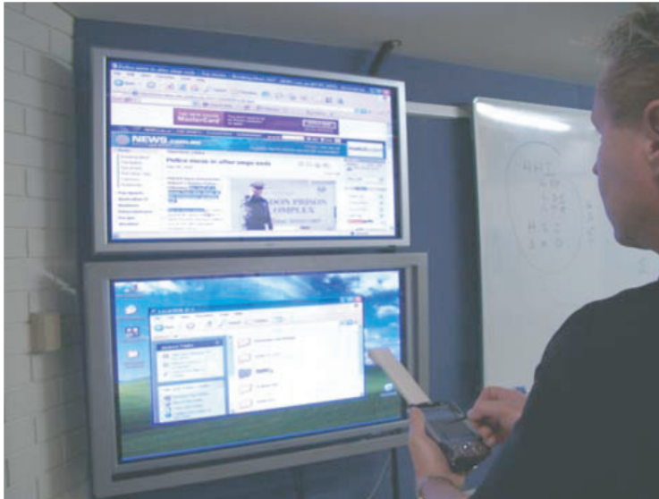
Figure 2.6: To interact with a room a user points her device to a display and uses the touch sensitive PDA to copy and paste content. Taken from [Slay and Thomas, 2006].
